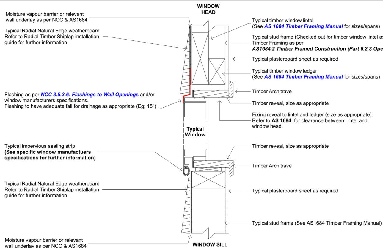
**NOTE: Window details are indication of cladding fixing only. For specific window flashing details it is recommended to refer to window manufacturers details**
