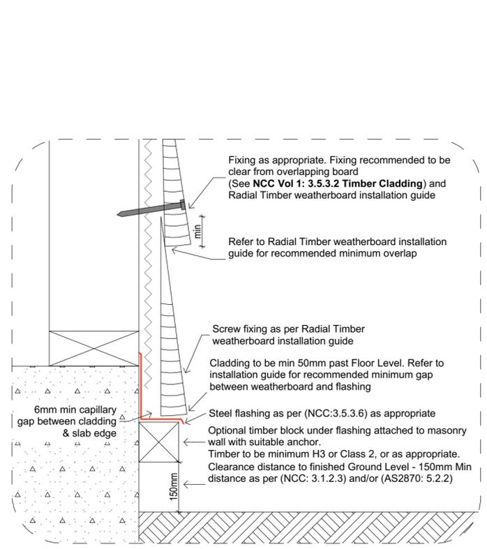
1.1 NE02:A1 - Radial Natural Edge Weatherboard - Bottom Flashing - Timber SubFloor
