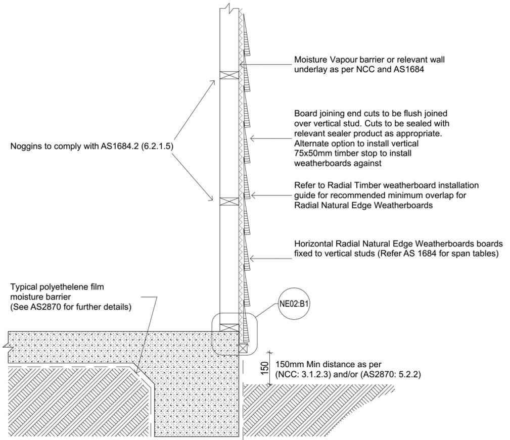
1.0 NE02:A - Horizontal Radial Natural Edge Weatherboard - Stud Frame: Timber Sub-Floor
