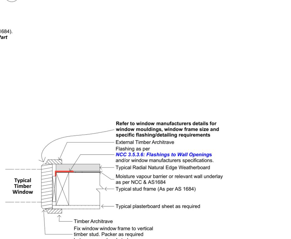
**NOTE: Window details are indication of cladding fixing only. For specific window flashing details it is recommended to refer to window manufacturers details**
